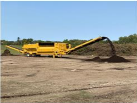
4. Compost material is run Through a trammel to Remove trash and other Inorganic material
